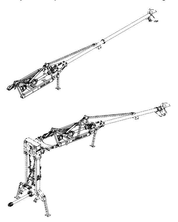
The slurry mixer adapter can be used between tractor and slurry mixer or between slurry mixer tower and slurry mixer.
